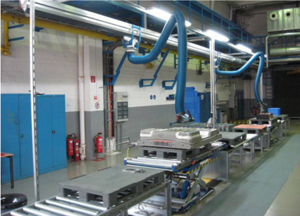
Figure 11. Dismantling of EDV Batteries at Umicore Facility in North Carolina, US
